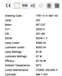
Input Voltage: 220-240Vac 50/60Hz
