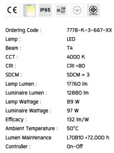
Input Voltage: 220-240Vac 50/60Hz
