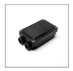
Ordering Code: AUN-DRG-0126-00 LED constant current driver, 250mA, 12W, with IP67 GFR polymer enclosure, On-Off, BLACK
