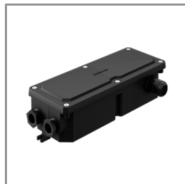
Ordering Code: AUN-DRG-0112-01 LED constant current decoder, 4x700mA, 4x23W, with IP67 GFR polymer enclosure, DMX512/RDM
