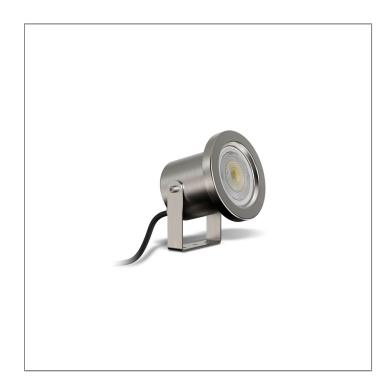
NIXIE is a range of stainless steel luminaires designed to be operated underwater. NIXIE Spotlight is made from 316 grade stainless steel and suitable for a wide range of low voltage retrofit LED lamps with GU5.3 socket. Equipped with a 1.5m long neoprene cable and epoxy potted cable entry. The spotlight is designed for permanent submersion in chlorinated swimming pools up to a depth of 1.5m.
