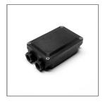
Ordering Code: AUN-COV-OOO2-OO LED constant current convertor input 12-24VDC, 700mA, 14W, with IP67 GFR polymer enclosure, On-Off
