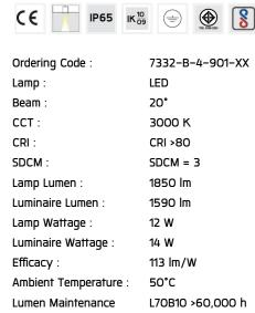
Input Voltage: 220-240Vac 50/60Hz
