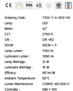
Input Voltage: 220-240Vac 50/60Hz
