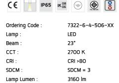
Luminaire Lumen : 3090 lm Lamp Wattage: 23 W Luminaire Wattage: 26 W 118 lm/W Efficacy: Ambient Temperature : 50°C
