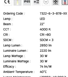
Lumen MaintenanceL70B50 >40,000 hController :On-Off [AC LED]Input Voltage :220-240Vac 50/60Hz
