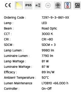
Input Voltage: 220–240Vac 50/60Hz
