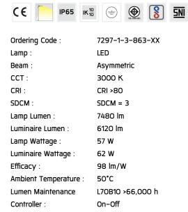
Input Voltage: 220–240Vac 50/60Hz
