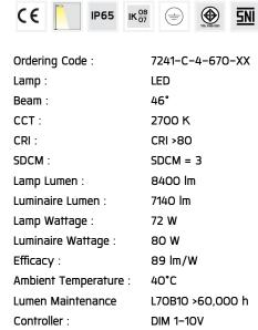
Input Voltage: 220-240Vac 50/60Hz
