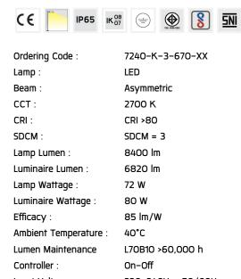
Input Voltage: 220-240Vac 50/60Hz
