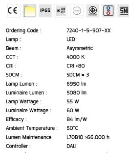
Input Voltage: 220–240Vac 50/60Hz
