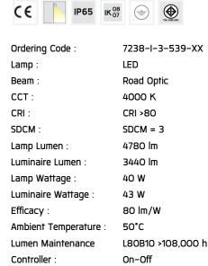
Input Voltage: 220-240Vac 50/60Hz
