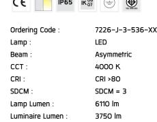
Lamp Wattage: 55 W Luminaire Wattage: 58 W Efficacy: 64 lm/W Ambient Temperature : 50°C
