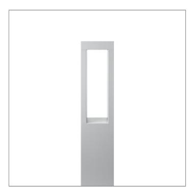
BICEPS is a family of luminaires designed for architectural spaces with functional low glare light output. Two different types of bollards and a light column make up the BICEPS family. The luminaires are suitable for pathways, parks, commercial areas and open spaces. Manufactured from corrosion resistant aluminum extrusions and a specially formulated LM6 aluminum alloy [LM6+], BICEPS is suitable for harsh environments.
