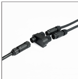
Ordering Code: AUN-CON-0012-00 IP68 connection device 5 pole, cable diameter 7.1-13mm, with distribution block , 1-10V or DALI
