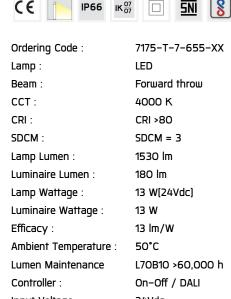
Input Voltage: 24Vdc Net Weight: kq.
