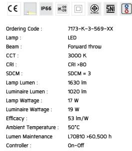
Input Voltage: 220-240Vac 50/60Hz
