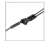
Ordering Code: AUN-CON-0010-00 IP68 Water Tight Connecting Device with Distribution block, 3 pole, 1 input, 2 outputs, Cable Diameter 5.0 - 9.5mm.
