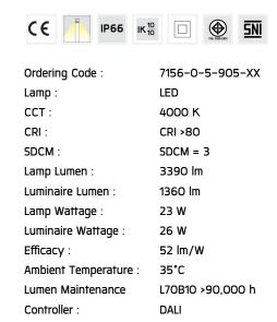
Input Voltage: 220-240Vac 50/60Hz
