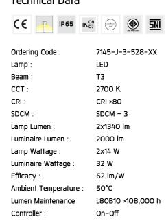
Input Voltage: 220–240Vac 50/60Hz
