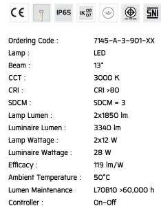
Input Voltage: 220-240Vac 50/60Hz
