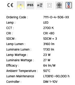
Input Voltage: 220-240Vac 50/60Hz
