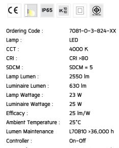
Input Voltage: 220-240Vac 50/60Hz
