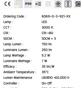
Input Voltage: 220–240Vac 50/60Hz
