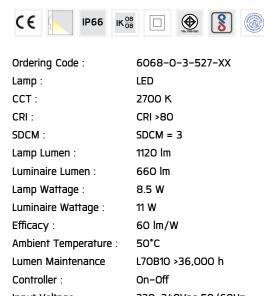
Input Voltage: 220-240Vac 50/60Hz
