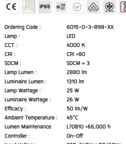
Input Voltage: 220-240Vac 50/60Hz
