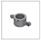
Ordering Code: AUN-CLP-OO46-XX Pole clamp, pole diameter 102-105mm, double sided luminaire mounting , On-Off, pre-assembly from factory
