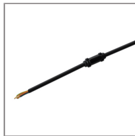
Ordering Code: AUN-CAB-0002-00 Cable H07RN-F 3x1sqmm, L= 2000, with UniBlock anti-humidity kit, pre-assembly from factory
