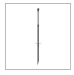
Ordering Code: AUN-ESP-0024-XX Earth spike, L= 1390-1760mm, aluminum, length adjustable, 1-10V or DALI, pre-assembly from factory
