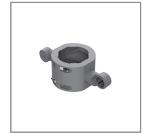
Ordering Code: AUN-CLP-O046-XX Pole clamp, pole diameter 102-105mm, double sided luminaire mounting , On-Off, pre-assembly from factory
