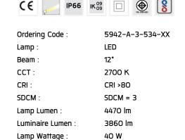
Luminaire Wattage: 89 lm/W Efficacy: Ambient Temperature : 50°C
