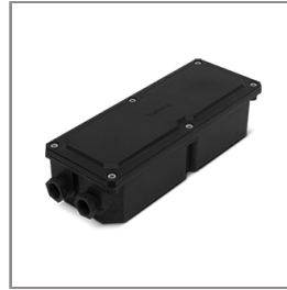
Ordering Code: AUN-DRG-0004-01 LED constant current driver, 1050mA, 22W, with IP67 GFR polymer enclosure, On-Off
