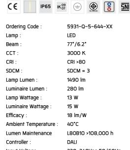
Input Voltage: 220-240Vac 50/60Hz
