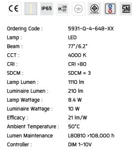
Input Voltage: 220–240Vac 50/60Hz
