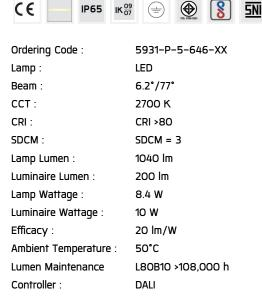
Input Voltage: 220-240Vac 50/60Hz
