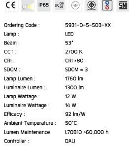
Input Voltage: 220-240Vac 50/60Hz
