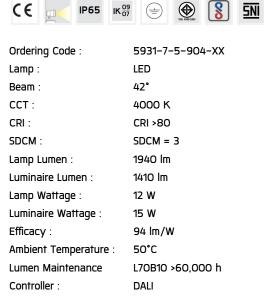
Input Voltage: 220-240Vac 50/60Hz
