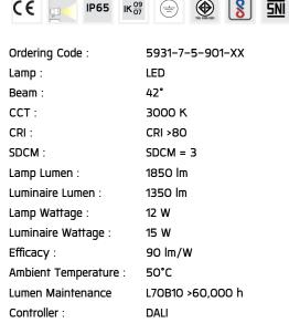
Input Voltage : 220–240Vac 50/60Hz
