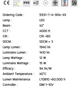
Input Voltage: 220-240Vac 50/60Hz
