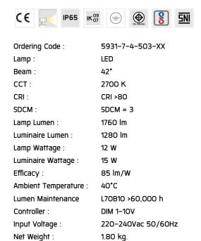
Ordering code guide XXXX-X-X-XXX-XX À Product Code Reflector Electrical Component C D Lamp Color
