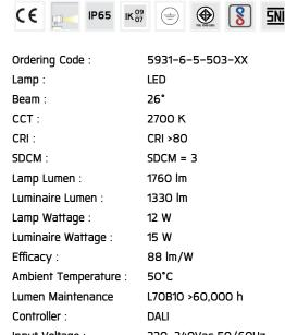
Input Voltage: 220-240Vac 50/60Hz
