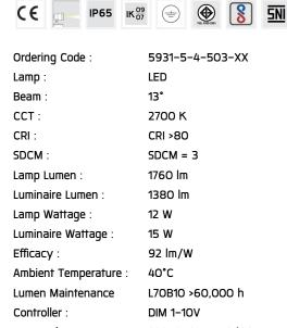
Input Voltage: 220-240Vac 50/60Hz
