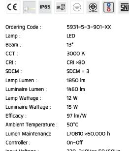
Input Voltage: 220–240Vac 50/60Hz
