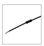
Ordering Code: AUN-CAB-0001-00 Cable H07RN-F 2x1sqmm, L= 2000, with UniBlock anti-humidity kit, pre-assembly from factory
