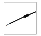
Ordering Code: AUN-CAB-0003-00 Cable 3x1sqmm and 2x0.35 sqmm length 2000 mm with anti-humidity kit. [pre-assembled from factory]
