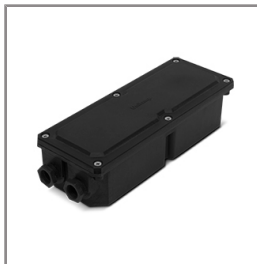
Ordering Code: AUN-DRG-0021-00 LED constant current driver, 1050mA, 38W, with IP67 GFR polymer enclosure, 1-10V
